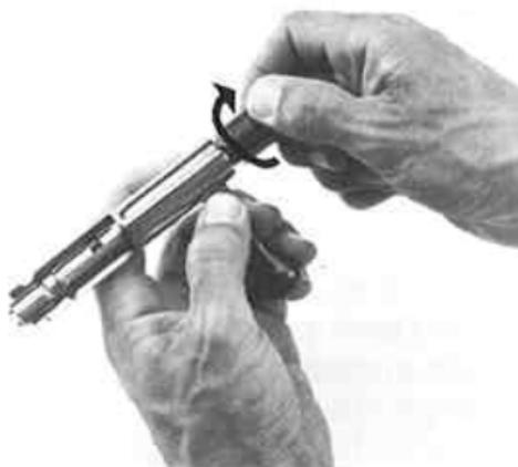
2. To be able to take off the bolt it would be the best to put it on the edge of a table or the like. (Figure 2).
